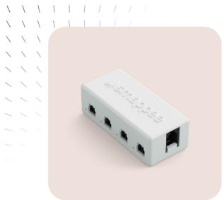
The CT Hub is the main component of the Smappee Infinity monitoring system. You can connect up to 4 Current Transformers (CTs) or Rogowski coils to a CT Hub to measure different currents up to 10,000 A. This allows for accurate submetering of (a group of) appliances. Daisy chain several CT Hubs to measure different installations up to a distance of 100 meters (109 yards).
