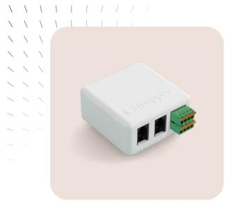
The Smappee Input module can count pulses of up to four digital inputs such as sensors, meters and other devices. It can also monitor state changes (low/high) to trigger other processes. Add up to 10 input modules to the Smappee Infinity setup thanks to its RJ10 connection. The modules transfer all collected data to the Smappee Genius. This data is available in the Smappee App, Dashboard and API.
